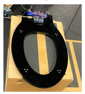
**Figure 1**: The instrumented toilet seat prototype. Four force sensors (with a max loading of 50kg) are placed between the seat and the ground, bearing the full weight of the participant. The sensors are individually measured, allowing for careful comparison of forces between each of the four locations to determine center of pressure and weight magnitude.
