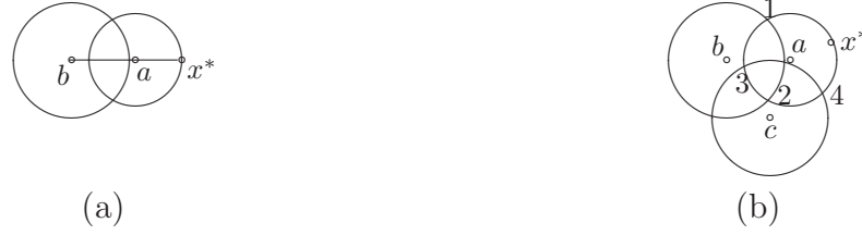
Figure 3.4: (a) Sensor with one anchor connection a and one neighboring anchor b . (b) Sensor with one anchor connection a and two neighboring anchors b, c .
