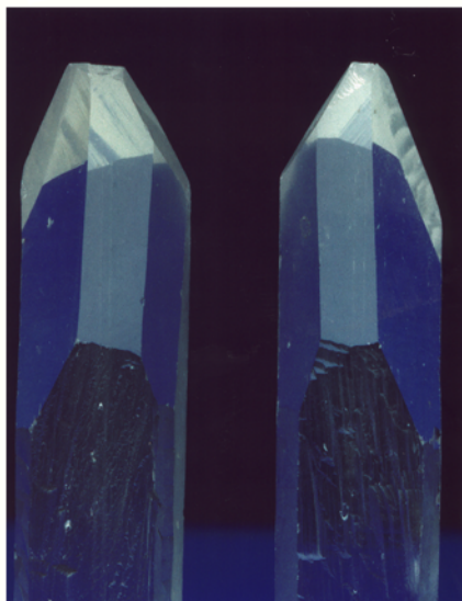
Fig. 11.2 Single crystals of morphologically enantiomeric quartz. Note the mirror symmetry of the facets on the respective crystals. Unlike amino acids, the component silicon dioxide molecules have no chirality. The spontaneous resolution of quartz into crystals of opposite morphological handedness is an example of local symmetry breaking in the environment.
