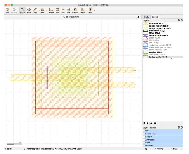
This refractive index for the areas specified with polygons with later be given the value of *foreground\_in-dex*. The image below illustrates the concepts of the layers and foreground and background indicies.
