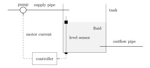
Note that when the outflow is equal to the known value  $Q_0$ , and the pump current is equal to its normal operating value, the supply flow is also equal to  $Q_0$ , so the net fluid flow into the tank is zero. This means the tank level remains constant, *i.e.*, half full.
