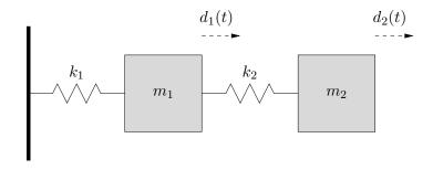
This two mass system is governed by Newton's equations of motion, which are
