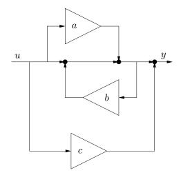
The triangle shaped blocks represent scaling systems with gains a, b, and c.
