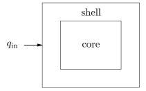
An external heat flow  $q_{\rm in}$  (in W) flows into the shell, and in addition there in a heat flow  $k_{\rm shell}T_{\rm shell}$  from the shell into the surroundings, where  $k_{\rm shell}$  is the thermal conductance between the shell and the surroundings.
