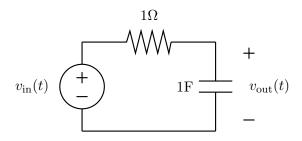
39. In the circuit below,  $v_{\rm in}(t)=1-e^{-2t}$  for  $t\geq 0$ , and the capacitor is uncharged at t=0. Find  $v_{\rm out}(t)$  for  $t\geq 0$ .
