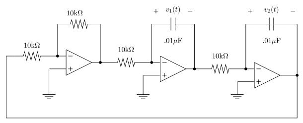
29. An RCRC circuit. Consider the circuit shown below. For t < 0,  $v_{\rm in}(t) = 1$ V and the circuit was in static conditions. For  $t \ge 0$ ,  $v_{\rm in}(t) = 0$ V.
