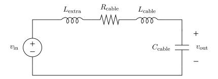
A second engineer responds: "Adding inductance is crazy! It's precisely the inductance that slows the cable, by fighting changes in current. Adding inductance will make the cable system slower, *i.e.*, decrease the decay rate."
