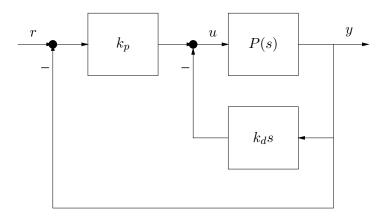
We'll study PD control applied to a DC motor, with transfer function
