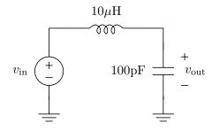
Find the transfer function H from  $v_{\text{in}}$  to  $v_{\text{out}}$ . (You can assume, of course, that the initial conditions are zero.)
