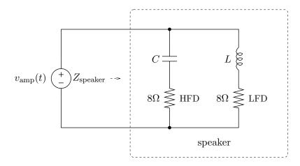
The crossover network is designed so that the transfer function from the amplifier to each driver has magnitude -3dB at a frequency  $\omega_c$  called the crossover frequency of the speaker.
