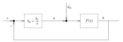
Some industrial PI controllers use the modified PI controller shown below:
