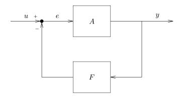
The open-loop gain A varies over the range  $60 \pm 3 \text{dB}$ . The closed-loop gain G varies over the range  $40 \pm \Delta \text{dB}$ .
