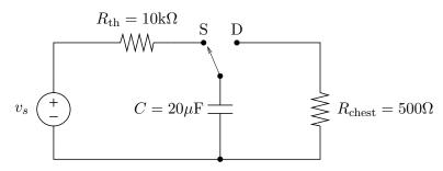
With the switch in the standby mode, indicated as 'S', the  $20\mu$ F capacitor is charged up by a power supply represented by a Thevenin voltage  $v_s$  and Thevenin resistance  $R_{\rm th} = 10 {\rm k}\Omega$ . When the switch is thrown to 'D' (for 'defibrillate'), the capacitor discharges across the
