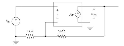
How much can the closed-loop gain (from  $v_{\rm in}$  to  $v_{\rm out}$ ) vary, taking into account both the variation in op-amp gain and the resistor variation? Which causes more variation in closed-loop gain, the variation in op-amp gain or the resistor values?
