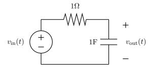
55. Reducing the rise-time of a signal. In a certain digital system a voltage signal should ideally switch from 0V to 5V infinitely fast, i.e., with zero rise-time. But due to the finite bandwidth of the electronics that generates the signal, it has the form
