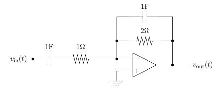
Find the DC gain, poles, and zeros of the transfer function from  $v_{\rm in}$  to  $v_{\rm out}$ . If the poles and/or zeros ar repeated, be sure to give the multiplicity.
