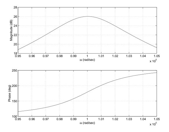
Estimate the poles, zeros, and DC gain of the transfer function H. Give the DC gain as a number, not in dB.
