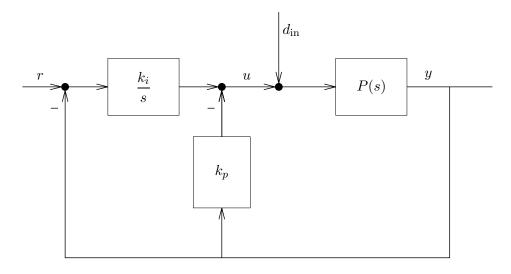
One company that makes this modified PI controller claims that it "has the same disturbance rejection abilities as the standard PI controller, but, for step changes in r, has a smoother input u".
