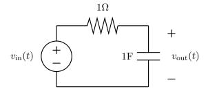
Find the output voltage,  $v_{\text{out}}(t)$ , for  $t \geq 0$ .
