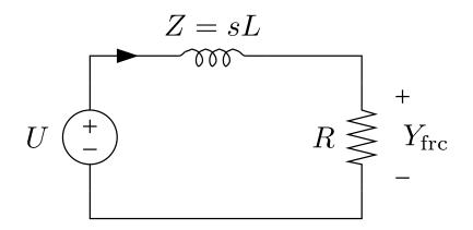
by voltage divider rule (for impedances),  $Y_{\rm frc}=U\frac{R}{R+sL}$  (as if they were simple resistors!)
