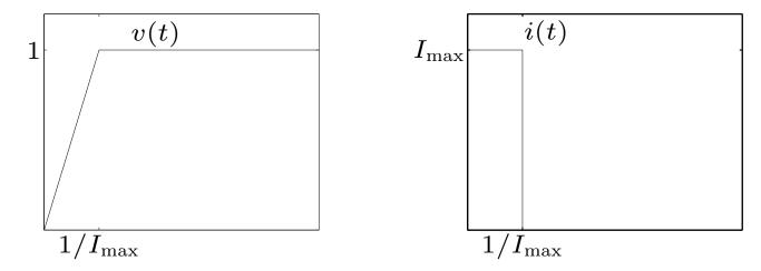
as  $I_{\max} \to \infty$ , i approaches an impulse, v approaches a unit step
