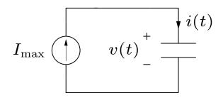
$$i(t) = \frac{dv(t)}{dt} = I_{\text{max}}, \quad v(0) = 0$$
