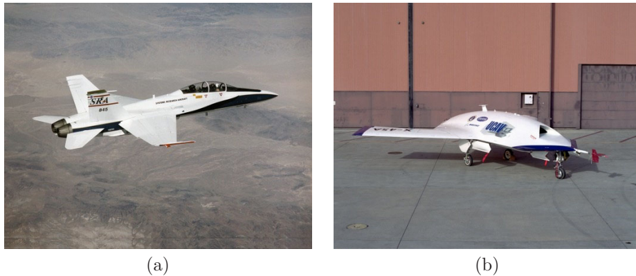
Figure 3.1. (a) The F-18 aircraft, one of the first production military fighters to use “fly-by-wire” technology, and (b) the X-45 (UCAV) unmanned aerial vehicle. Photographs courtesy of NASA Dryden Flight Research Center.
