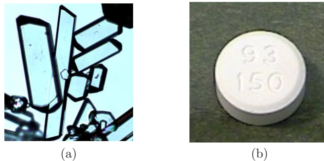
Figure 3.12. (a) Microscope image of paracetamol crystals (paracetamol is the active ingredient in Tylenol (b)), which shows the variability in crystal shape that can occur at a single time instance in a pharmaceutical crystallizer. Image courtesy of Richard Braatz.
