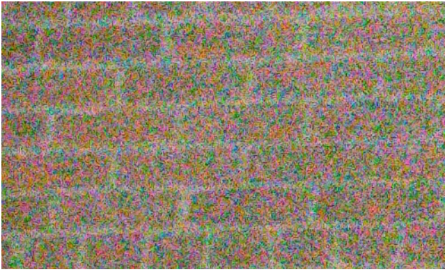
Figure 2: A raw frame captured in daylight with a Nexus 5 rear camera (after demosaicking). The image was taken at ISO 3000 with a 30 ms exposure time. The noise in the image is clearly visible.
