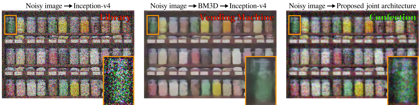
Figure 1: The performance of deep networks trained for high-level computer vision tasks such as classification degrades under noise, blur, and other imperfections present in raw sensor data. (Left) An image of jelly beans corrupted by noise characteristic of low-light conditions is misclassified as a library by the Inception-v4 classification network. Cleaning up raw data using conventional low-level image processing does not necessarily improve performance. (Center) The image denoised with BM3D is still misclassified, now as a vending machine. We propose an end-to-end differentiable architecture for joint denoising, deblurring, and classification that makes classification robust to realistic noise and blur. The proposed architecture learns a denoising pipeline optimized for classification that enhances fine detail at the expense of more noise and artifacts. (Right) The learned denoiser recovers the jellybean texture, and the image is correctly classified in the “confection” category. The proposed architecture has a principled and modular design inspired by formal optimization methods that generalizes to other combinations of image formation models and high-level computer vision tasks.
