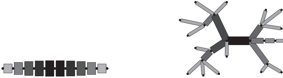
Fig. 5 Left: Optimal conductance allocation on a path on 11 nodes. Right: Optimal conductance allocation on a tree with 25 nodes.
