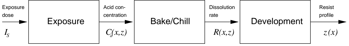
Figure 1. The manufacturing steps relevant for design of optimal temperature profiles.
