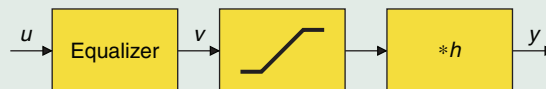
[FIG5] Our pre-equalizer processes the incoming signal u (with a look-ahead of T samples), to produce the input, v , applied to the system.
